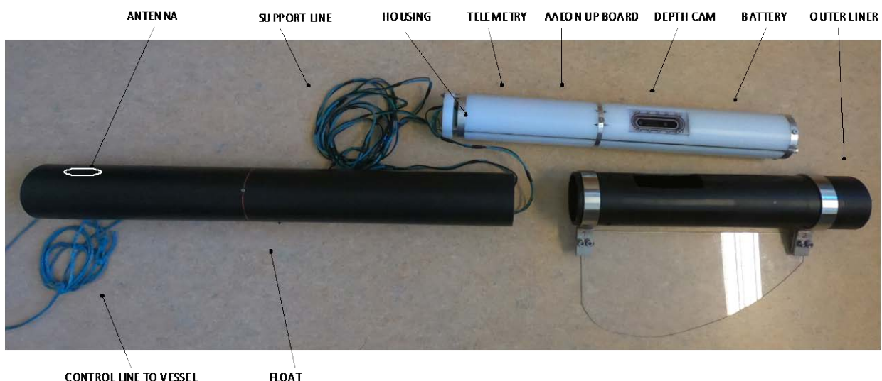
Figur 6. Oversikt over deler i Stereo Catch Monitoring Probe (S-CMP).
